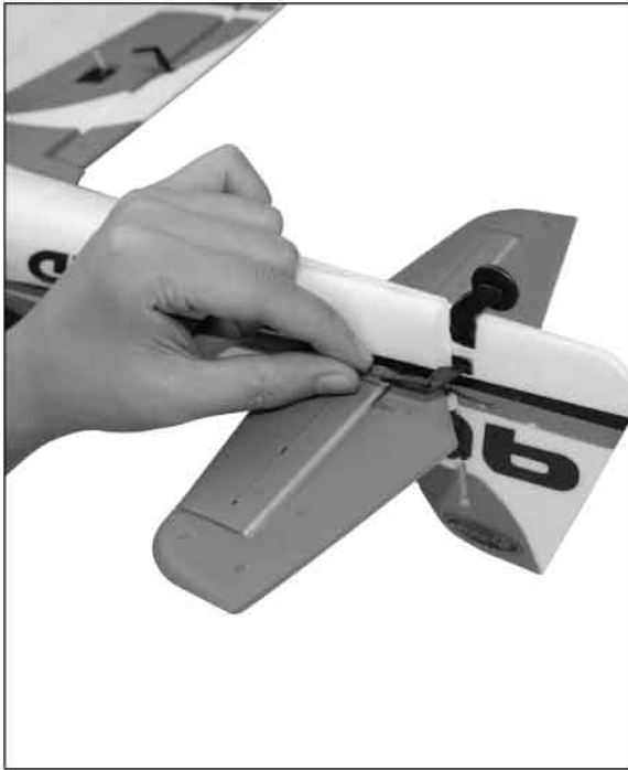
5 Install rudder push rod as shown.
