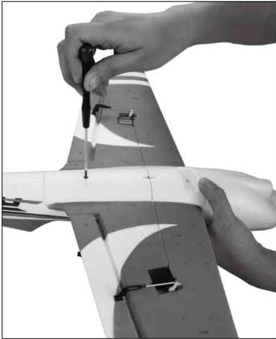
1 Fix the wing with PM3*25mm screw.
