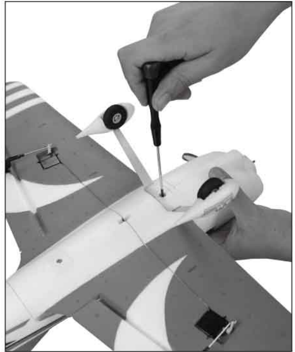
2 Install the landing gear with PM3*25mm screws.
